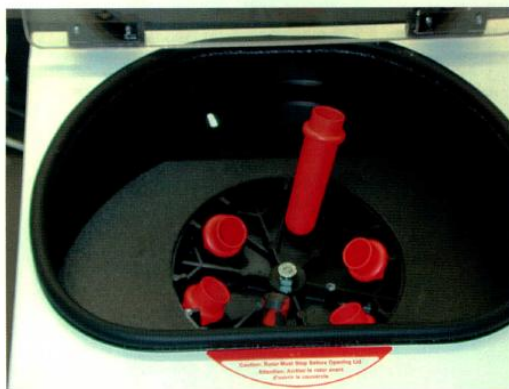
Figure 28.21 Removable centrifuge sleeves should be sterilized for each case.
