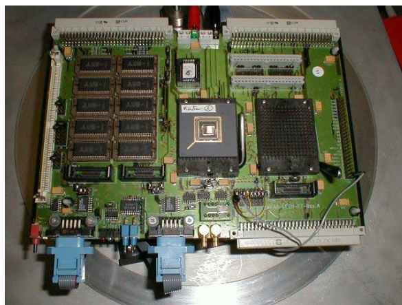
Figure 5: LEON-Express SEU test board
