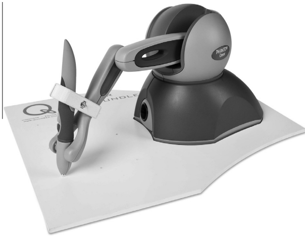
Fig. 3. The PHANTOM Omni device used in our experiments [25].
